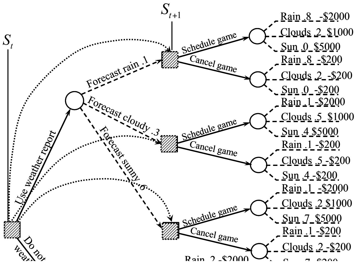
$$V_t(S_t) = \max_{x \in X} \left( C_t(S_t, x_t) + E \left\{ V_{t+1}(S_{t+1}) \mid S_t \right\} \right)$$
