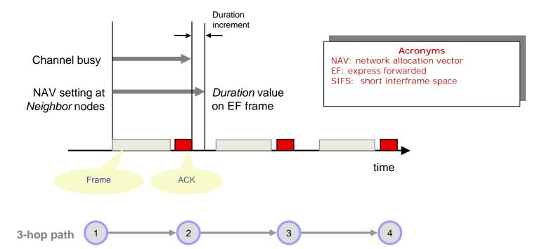
The Duration field of an EF frame is set at value longer than usual when it is transmitted to a forwarding node of a multi-hop path; the Duration increment is
